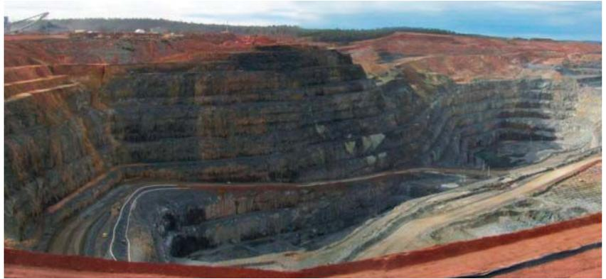
▲ **NEWMONT BODDINGTON PIT**, 900 feet deep and going deeper all the time, creates difficulties for GNSS equipment positioning the mine's heavy machinery.
