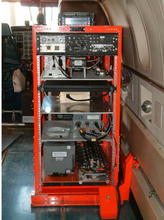
IMAGE 2: The current USAF “truth system” rack, against which a 5-inch square Locata receiver was directly compared.
