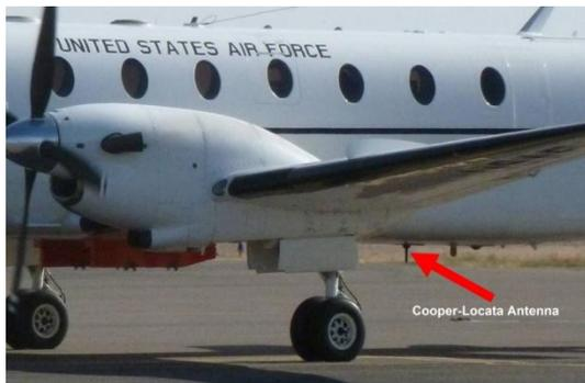
**Figure 7 Antenna Mounted on C-12J**
