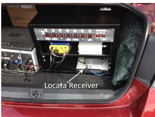
**Figure 6: A Locata Receiver, installed as an integral part of the DAK, provides position accuracy to <10cm**
