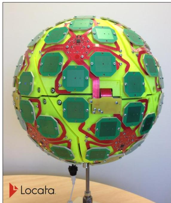
**Locata VRAY Orb-80 Antenna:** The first commercial VRAY antenna, designed to mitigate multipath for difficult machine automation applications in warehousing, supply-chain, port and industrial environments. This design will be modified by AFIT for use with GPS receivers.
