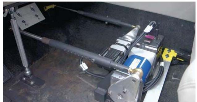
▲ **DROP-IN ACTUATOR KIT** steering (top) and throttle-brake (bottom).
