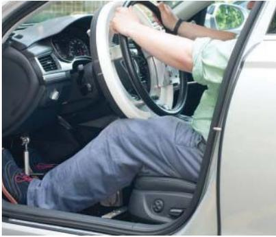
▲ A HUMAN OPERATOR is easily accommodated within the drop-in actuator kit.
