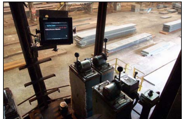
Figure 5. View from crane drivers cab with VDU for job instructions.
