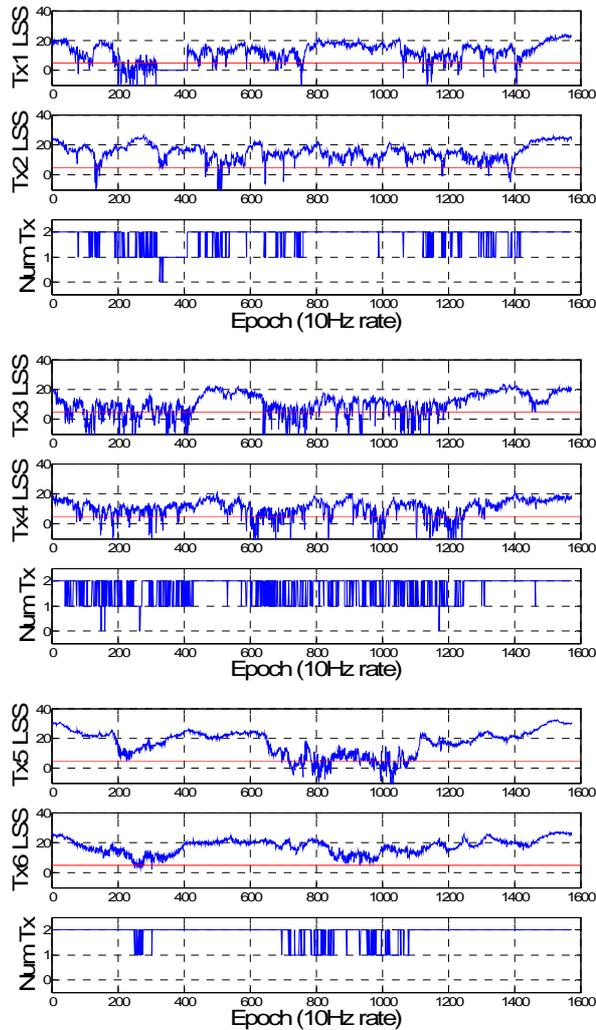
Fig. 10. Example LSS and Tx count for *LocataLites* 1/2, 3/4, 5/6
