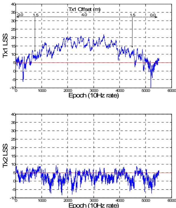
Fig. 5. Spatial diversity experiment results: LSS values for Tx1 and Tx2.
