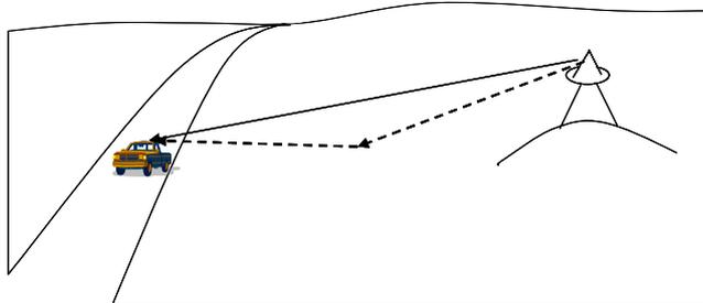
Fig. 1. Illustration of low incident multipath reflections for any terrestrially-based RF positioning system,
