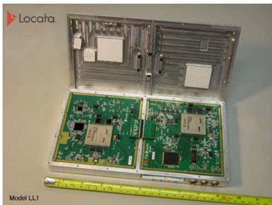
Figure 2. *LocataLite* (transceiver) hardware.
