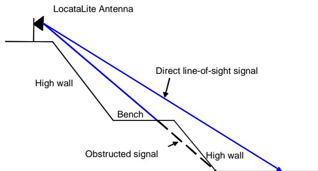
**Figure 12.** Obstructed LocataLite signal close to high wall.
