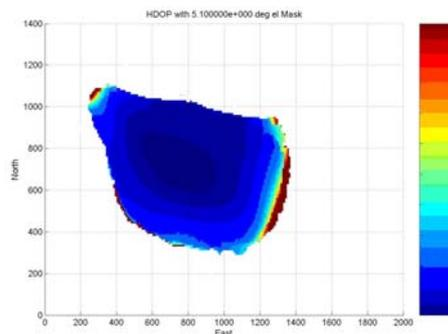
**Figure 3.** Expected horizontal dilution of precision from LocataNet.
