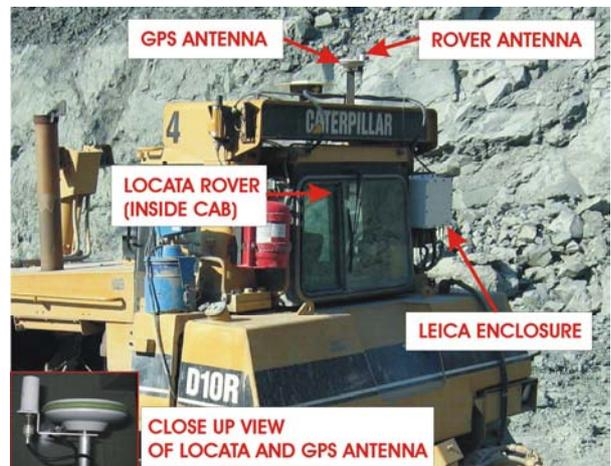
**Figure 7.** Dozer installation
