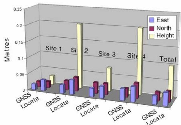
**Figure 15.** GNSS RTK and Locata Backpack RMS statistics.
