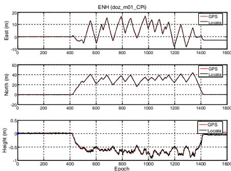
**Figure 16.** Dozer session: GNSS versus Locata position solution.
