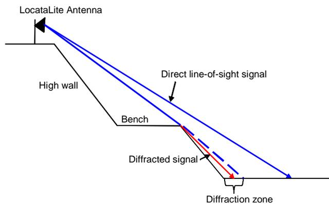
**Figure 13.** Diffracted LocataLite signal close to high wall.
