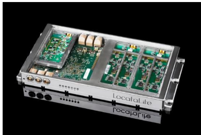
Figure 1-1: Locata Transmitter – LocataLite (with top cover removed)
