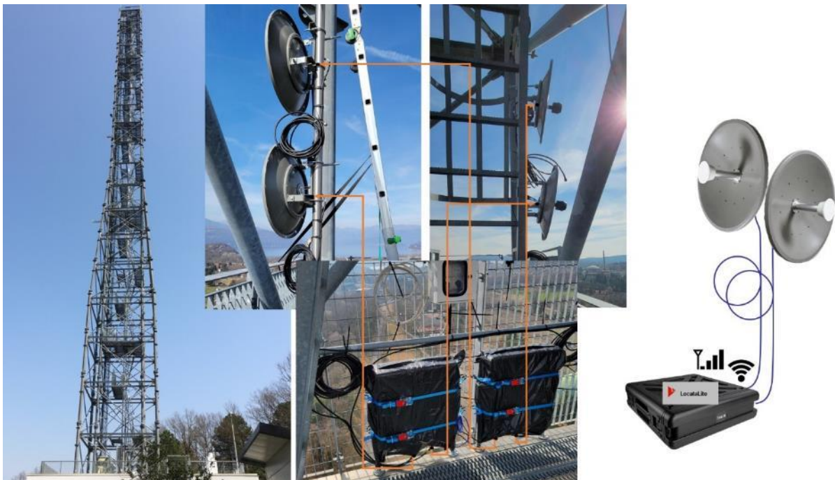
Figure 3-2: LocataLite Setup with Dish Antennas at the JRC Tower for Wide Area Time Transfer
