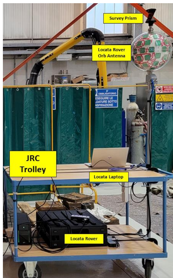
Figure 4-6: Locata Rover Setup with Locata VRay Orb Antenna for Indoor Positioning Test
