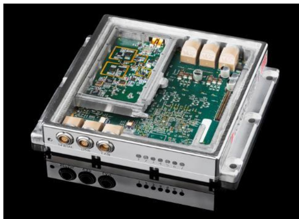
Figure 1-2: Locata Receiver – a Rover (with top cover removed)
