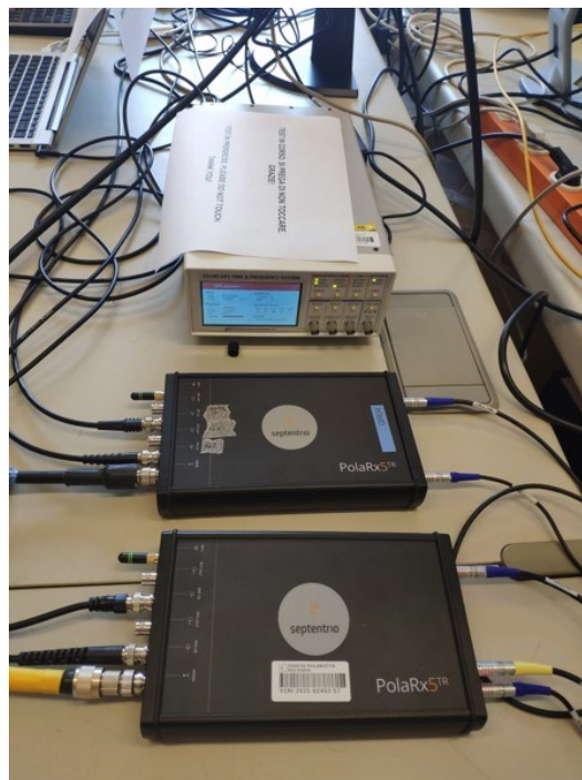
Figure 5. Calibration setup, JRC time reference visible on top
